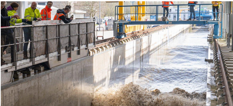
A clay ripening project demonstrates how (dredged) sediment can be converted to clay soil for dike reinforcements. Levee of ripened clay tested in the Delta Flume at Deltares.
